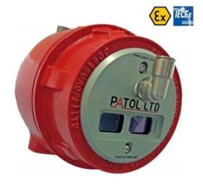
The 5710 High Temperature Transit Flame Sensor monitors high temperature materials (up to 240° on highest sensitivity), being transported on conveyor systems at speeds of between 0.5 and 6m/s, and triggers as the material reaches the ember or flame condition.
